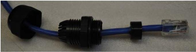
The next step is to push the rubber ring into position so that it will compress when the gland is assembled. You should GENTLY use a small screwdriver to slide it inside the main body of the gland housing until it is flush with the little plastic fingers at the bottom of the gland, like shown in the picture to the right->
